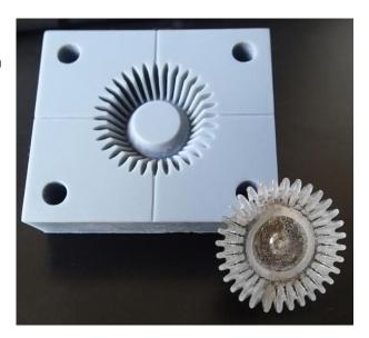
Thermal degradation of the 3D-printed mold has not been observed in any of the tests. Polymers like ABS, PA6 and PA12 show adhesion to the mold, while other polymers like PP, PE, HDPE and PETG release easily from the mold and are compatible with Strong-X 3D-printed molds. The test results were obtained with the use of two three-dimensional molds from Strong-X, and therefore a mirror plate is not used. Over 100 injections were successfully done with HDPE, PE and PP.
