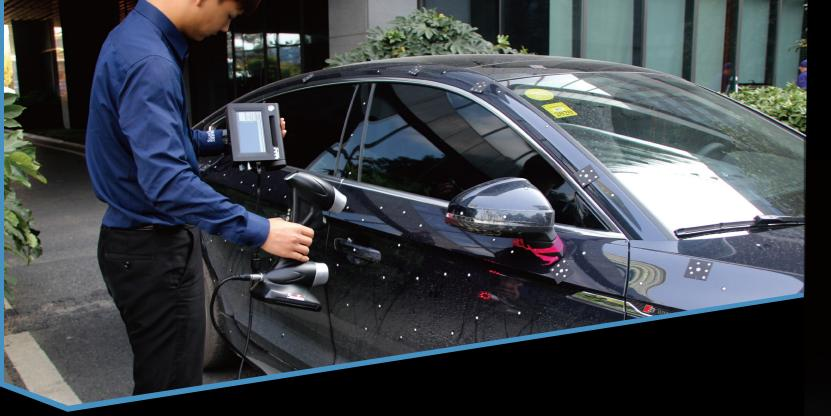
AirGO completely breaks through traditional 3D scanning methods and gets free from PC and cables. It can display 3D model directly on hand and truly perform efficient as well as flexible 3D measurement.
